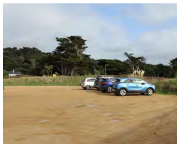
Crushed stone or hoggin are generally more suitable than metalled surfaces for rural car parks and access tracks
